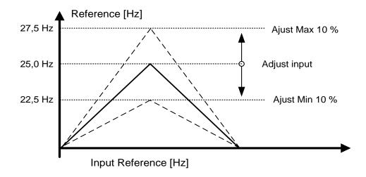
If minimum and maximum are not equal to zero, the adjustment is not at the middle point of analogue input or at zero point in case -10...+10 Vdc input is used. In the below picture, the minimum is 20% and the maximum 10%.
