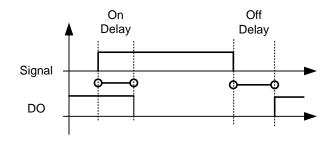
Select the signal for controlling the DO. The parameter has to be set in format xxxx.yy where xxxx is the ID number of a signal and yy is the bit number. For example, the value for DO control is *1174.02*. 1174 is the ID number of Warning Word 1. So the digital output is ON when bit number 02 of the warning word (ID no. 1174) i.e. *Motor underload* is high.
