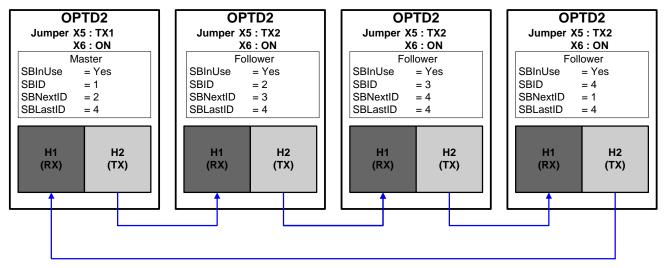
Figure 7-16. System bus physical connections with the OPT-D2 board
