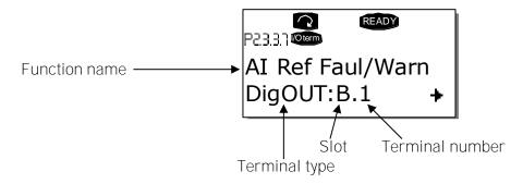
**Example**: You want to connect the digital output function *Reference fault/warning* (parameter 2.3.3.7) to the digital output DO1 on the basic board NXOPTA1 (see VACON® NX User Manual).
