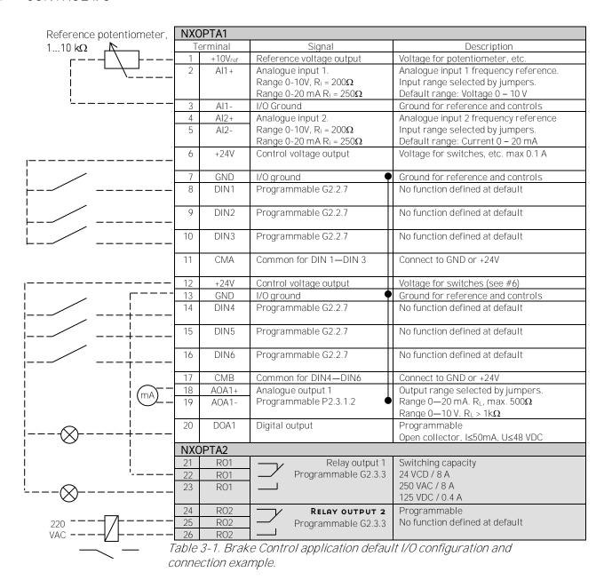
Note: See User Manual, chapter Control Connections, for hardware specification and configuration.
