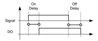
Figure 7-11. Digital outputs 1 and 2, on- and off-delays
