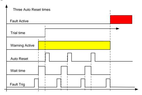
Figure 7-18. Example of Automatic restarts with three restarts
