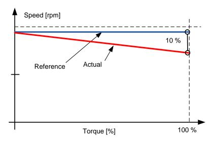
**Example:** If load drooping is set to 10% for a motor that has a nominal frequency of 50 Hz and is nominally loaded (100% of torque), the output frequency is allowed to decrease 5 Hz from the frequency reference. The function is used for e.g. when balanced load is needed for mechanically connected motors.
