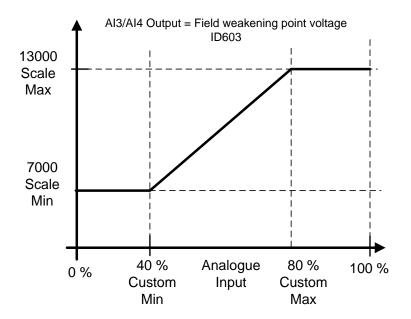
Now analogue input 3 signal 0 V to 10 V (0 mA to 20 mA) will control the field weakening point voltage between 70.00%–130.00%. When setting the value remember that decimals are handled as integers.
