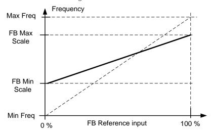
Using this custom scaling function also affects the scaling of the actual value.
