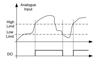
Figure 7-13. An example of On/Off-control
