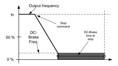
Figure 7-15. DC-braking time when Stop mode = Ramp
