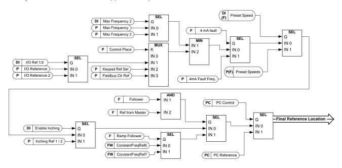
Speed reference chain before ramp control
