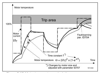
Figure 7-17. Motor temperature calculation
