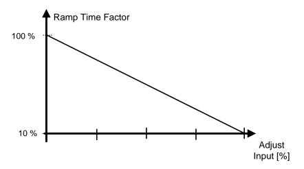
Figure 7-4. Reducing acceleration and deceleration times
