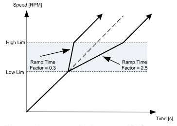
Figure 7-1. Ramp rate scaling between prohibit frequencies
