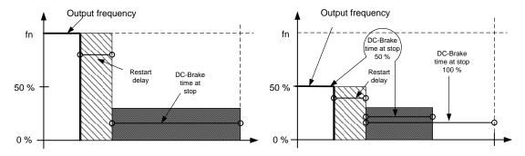
Figure 7-14. DC-braking time when Stop mode = Coasting, from nominal speed and 50% of nominal speed.
