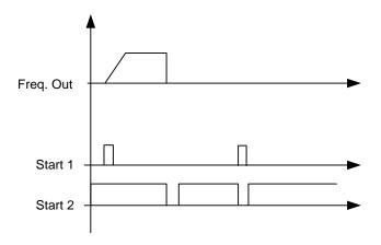
Figure 7-8. Start pulse/ Stop pulse.
